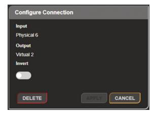
In this window the input and output link connects can be seen. There is also an option to invert the link which means that if the link would normally be off, it is instead on, and if a link would normally be on, it is instead off.
