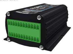
It has 10 configurable GPIO's, 8 of which can be used for PTP based programming, together with a relay. It provides virtual GPIO that allow the device to trigger or be triggered by other Sonifex devices on the network using virtual GPIO without the need for extra wiring (virtual GPIO communication occurs via the Ethernet connection).
